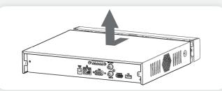
Step 2: Remove the case cover in the direction shown by the arrow above.
