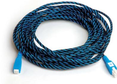
Each length of Hydrowire is terminated with a male and female 4 way plug to enable them to be plugged together up to maximum zone length of 50 metres and terminated with an EOL. It is connected to the panel through the Connection Interface. As soon as the cable detects moisture this will trigger an alarm. For the cable to measure water on the surface then it is recommended that the cable is fixed down with Hydrosense fixing clips (HY-FXSA)
