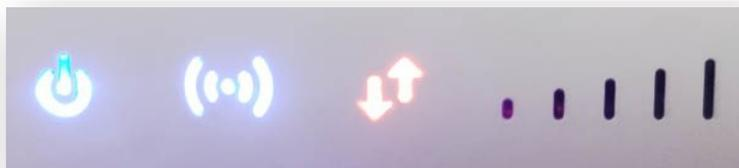
Once the correct APN has been entered and you reboot the device, wait for the red arrows to go blue and the signal level indicators to display. If there are no signal indicators lit, then your chosen SIM provider has no service in the area.
