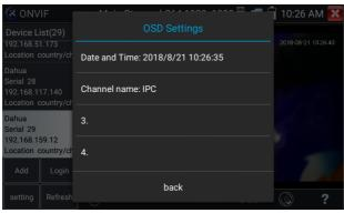
After selecting channel, you can edit the channel name, modify the display position, and switch the font size. If not modify, select "Content location - Default location". Select "Customize" to arbitrarily adjust the channel name and display location.
