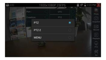
If to coaxial PTZ control the AHD camera, no parameters setting is needed.
