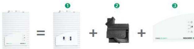
The aspirating smoke detector consists of the basic device (1), one or two detector modules (2) and an adhesive front film sheet (3).
